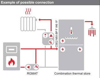
The diagram shows a typical connection of a solid fuel boiler (with the recommended RGMAT pump station – not included in supply), combination thermal store and heating circuit.
