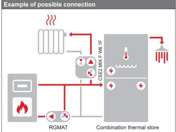
The diagram shows a typical connection of a solid fuel boiler (with the recommended RGMAT pump station – not included in supply), combination thermal store and heating circuit.
