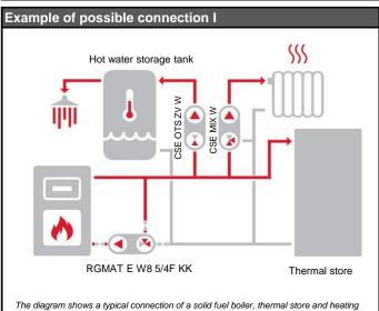
The diagram shows a typical connection of a solid fuel boiler, thermal store and heating circuit (with the recommended CSE MIX W pump station – not included in supply). If the boiler is used also for hot water heating, it is recommended to install a CSE OTS ZV W pump station (not included in supply).
