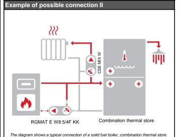
and a heating circuit (with the recommended CSE MIX W pump station – not included in
