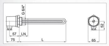
The elements feature a longer non-heating end (dimension LN) that permits their use for Regulus Thermal Stores with DHW.
