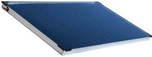
Flat plate collector of 1866 W output (at 1000 W/m<sup>2</sup> irradiance), designed for on-roof landscape installation. A harp absorber with highly selective TiNOx surface is laser welded to the copper pipes. The insulation consists of 40 mm mineral wool. Connections are located on both sides on the top.
