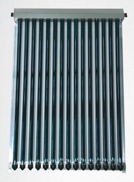
Evacuated tube collector of 1090 W output (at 1000 W/m² irradiance), designed for on-roof portrait installation. A tube consists of 2 coaxial glass tubes with vacuum between them. An aluminium lamella fitting closely to the glass tube collects heat from the whole inner surface of the evacuated tube, giving it away into solar fluid inside the copper pipe. These copper pipes join the collector header, insulated with 30 mm of mineral wool.
