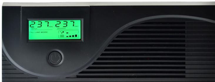
If the power supply cord is connected, press ON button and the PG 500 will work either in 230 V mode or in a battery mode, depending on whether the power supply is available. One more pressing the button will turn off the inverter control but the battery charging is maintained (supposed the incoming 230 V power is available).
