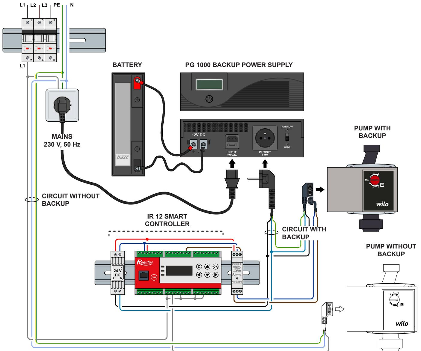
**!** Do respect the separation between the circuits with and without backup. Not only for the live wire but also for the neutral one!
