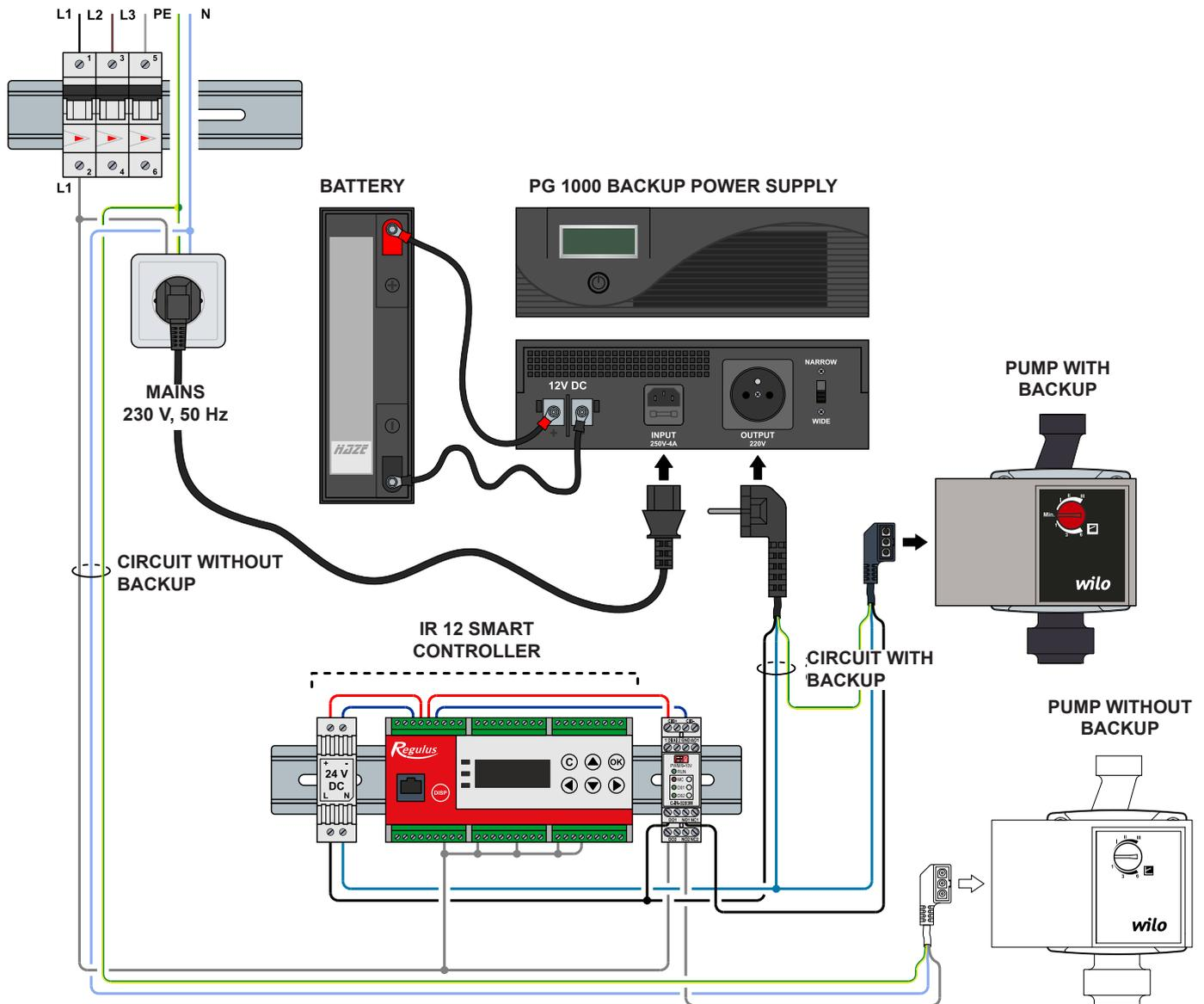
**!** Do respect the separation between the circuits with and without backup.
