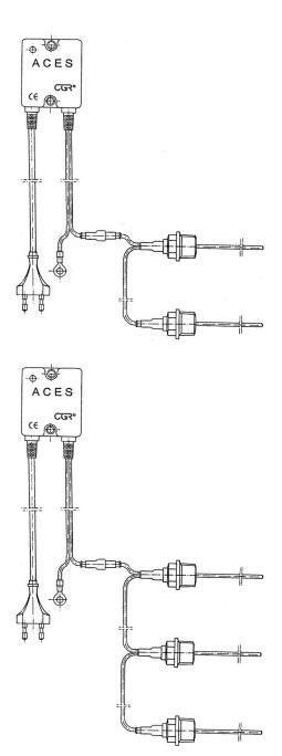
ACES, assembled with cables and two, three anodes.
