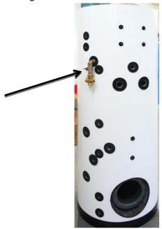
6. Loosen the clamps, fit the metal sheet against the four pins, code 12710 from Kit code 12224, and fix using 4 screws M6x16 with washers (codes 12996 and 7853) - both these components are included in the Kit code 13485. Do not forget to place insulation washers under and on the metal sheet. The single-circuit variant is fitted with the left clamp only.
