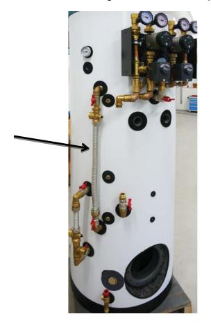
20. Locate the 1" hex nipple (in the pump station with 4-way mixing valves) fitted as shown in point 9 and the 1" Valve Assy fitted as shown in point 11. Connect these two using the dedicated 1" pipe, 690 mm long, code 13489.
