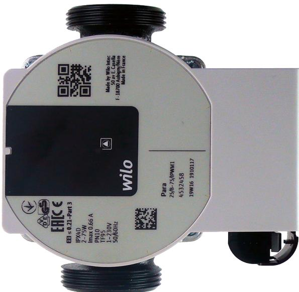
The Wilo Para 25/8 iPWM1 is a wet running circulation pump. The pump speed is controlled by the PWM signal. When the PWM signal is disconnected, the pump runs at its maximum speed. The operating status and possible faults of the pump are indicated by LEDs directly on the pump. The pump can send the current flow rate electronically to an external controller. The controller needs to be equipped with an iPWM read input and a flow rate calculation function.
