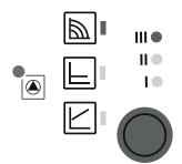
Briefly press the operating button for 1 second to select operating mode and pump performance curve. LEDs show pump settings (operating mode / performance curve).
