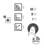
If the pump has been inactive for a long time or is blocked, activate the manual restart by holding the operating button for 5 seconds. The LEDs flash sequentially clockwise. The manual restart takes max. 10 minutes before the pump returns to normal operation. To cancel the manual restart, hold down the operating button for 5 seconds.
