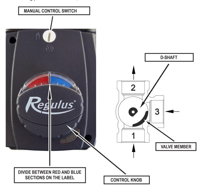
After the actuator is fitted, the correct position of the round indication label (hot/cold, red/blue) shall be checked as to the right function and position of the valve; the colours shall correspond to the cold and hot water connections. In case of a vertical installation in central heating, the red mark on the label shall be on the right-hand side for left-hand installations (see Fig. 5) and on the left-hand side for right-hand installations (see Fig. 6).
