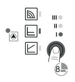
To lock the operating button, press it for 8 seconds.
