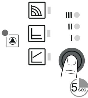
If the pump has been inactive for a long time or is blocked, activate the manual restart by holding the operating button for 5 seconds. The LEDs flash sequentially clockwise. The manual restart takes max.
