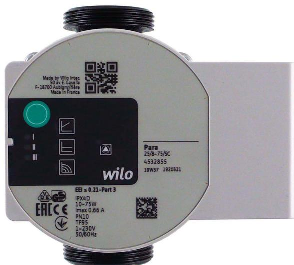
The high efficiency circulation pumps of the PARA SC series are used exclusively for the circulation of liquids in hot water heating systems. Operating the pump in other systems or in systems lacking water, containing air or in unpressurized systems can lead to its rapid destruction.
