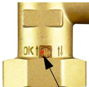
When the red mark is on the left-hand side, the non-return valve is set to normal operation position. If you need to open the valve (e.g. to drain the system), rotate its control so that the red dot is on the right-hand side. The non-return function is thus out of operation.
