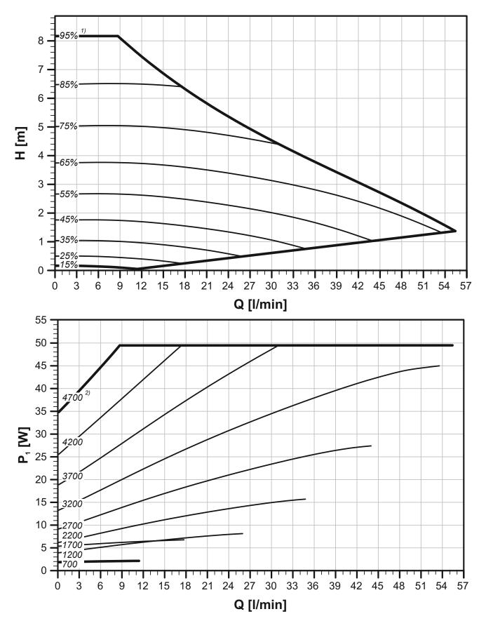
NOTE: 1) value of PWM signal in % 2) speed in rpm
