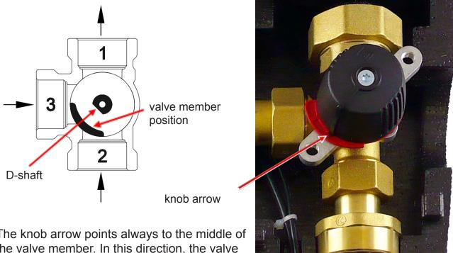
The knob arrow points always to the middle of the valve member. In this direction, the valve is closed.
