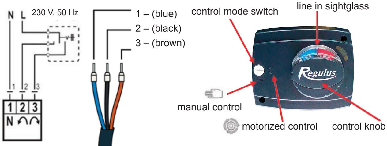
**The actuator is factory set to motorized control and ready for operation. Should it be inevitable to remove it or replace, please follow the instructions in the appendix.**
