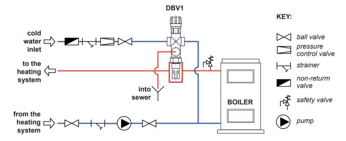
Pic. 3: Piping diagram for DBV1
