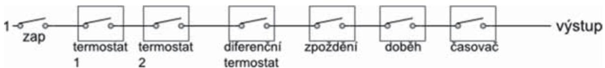
It is obvious from the picture that the Delay function can delay signal from thermostat and diff. thermostat functions, the Overrun function can hold disconnection (switching off) from thermostat, diff. thermostat and delay functions. The Timer function is superior over all the preceding functions.
