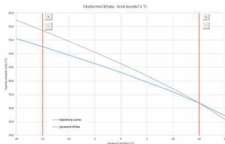
If a building overheats at an outdoor temperature below zero, the heating water temperature shall be reduced with the minus button. The graph shows that the heating water temperature will be adjusted mainly at temperatures below zero.
