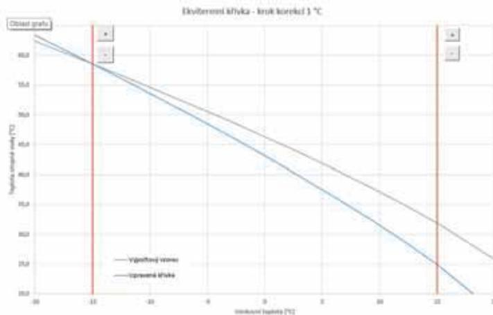
If a building overheats at an outdoor temperature above zero, the heating water temperature shall be reduced with the minus button. The graph shows that the heating water temperature will be adjusted mainly at temperatures above zero.
