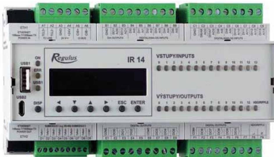
The keys **▲**, **▼** are used to browse in the menu. In order to edit a parameter, press **ENTER** and a cursor appears on the parameter. The values of numeric parameters can be increased/decreased by pressing **▲** / **▼** keys. Selection parameters (e.g. ON/OFF) are chosen by pressing keys **◀**, **▶**. When finished, pressing **ENTER** will move the cursor to the next parameter in the same display. Parameter editing can be also exited without saving by pressing the key **ESC**.
