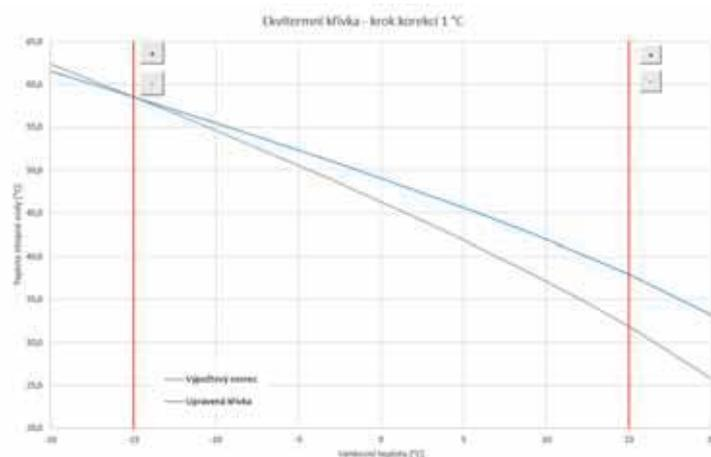
If a building underheats at an outdoor temperature above zero, the heating water temperature shall be increased with the plus button. The graph shows that the heating water temperature will be adjusted mainly at temperatures above zero.
