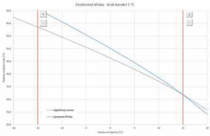
If a building underheats at an outdoor temperature below zero, the heating water temperature shall be increased with the plus button. The graph shows that the heating water temperature will be adjusted mainly at temperatures below zero.
