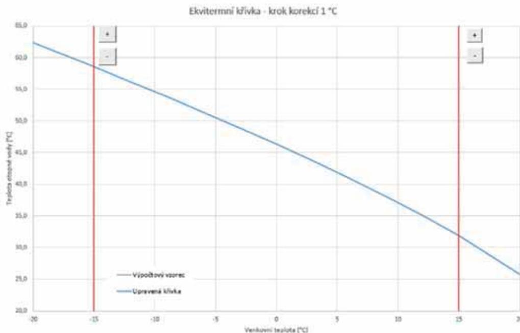
This model example shows a system with convection radiators with a temperature gradient of 55/50°C. The outdoor design temperature is -15°C, the indoor design temperature is 20°C and the desired indoor temperature is 22°C.
