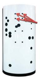
11. Fit the fresh water station (code either 9717 or 9913) using 4 screws M6x16 with washers (codes 12996 and 7853) - all these components are included in the Kit code 12226.
