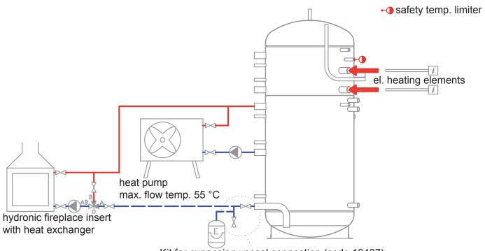
Kit for expansion vessel connection (code 13437). During operation, the 6/4" valve shall be secured in an open position.
