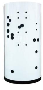
4. Peel off the protective foil from the insulation, apply the self-adhesive annuluses around the openings for connections. Some annuluses are cut out, these shall be used in places where openings are close to each other (the annuluses overlap).
