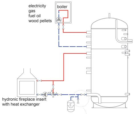
Kit for expansion vessel connection (code 13437). During operation, the 6/4" valve shall be secured in an open position.
