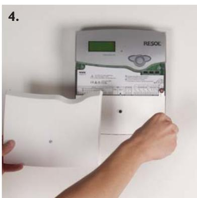
The unit must only be located internally. It is not suitable for installation in hazardous locations and should not be sited near to any electromagnetic field. The controller must additionally be equipped with an all-polar gap of at least 3 mm or with a gap according to the valid installation regulations, e.g. LS-switches or fuses. Please pay attention to a separate laying of the cable lines and installation of a power supply.
