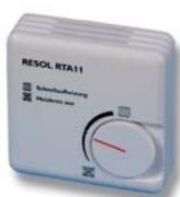
The remote control RTA11 allows a comfortable adjustment of the heating curve of the controller from the living room. The rise of the heating curve causes an increase in flow temperature, a fall causes a decrease. The remote control additionally contains the functions "heating circuit-off" and "fast heating-up".
