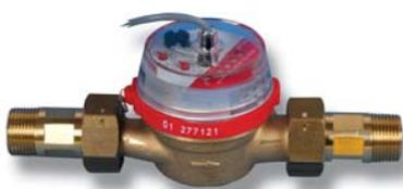
The RESOL V40 is a measuring instrument with contact donator for recording the flow of water or water/glycol mixtures and is used in combination with the calorimeter integrated into the DeltaSol M. After flow of a specific volume, the V40 sends an impulse to the calorimeter. The used heat amount is measured by these impulses and a measured temperature difference with the help of pre-defined parameters (glycol type, concentration, heat capacity, etc.).
