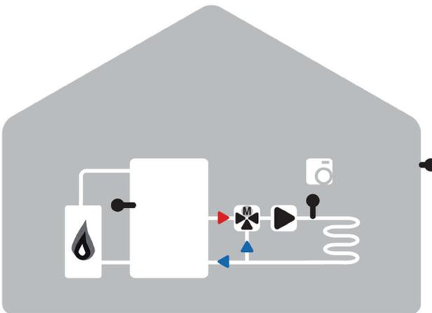
**4. Two heating circuits - mixed and direct one, no boiler, no accumulation tank**
