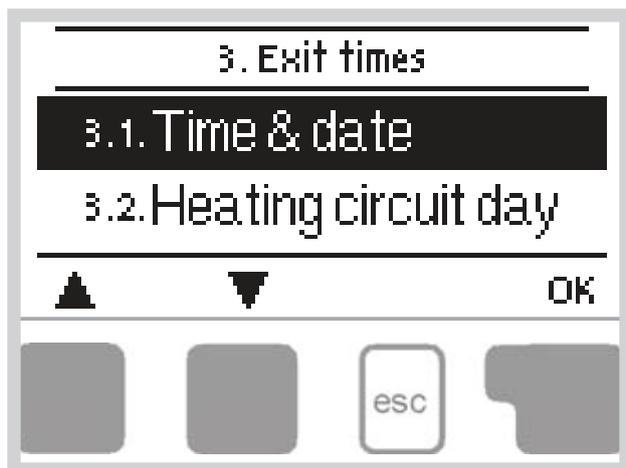
Menu „**3. Times**” is used to set the time, date and operating times for the heating circuit.
