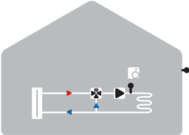
**2. Mixed heating circuit with boiler, no accumulation tank**
