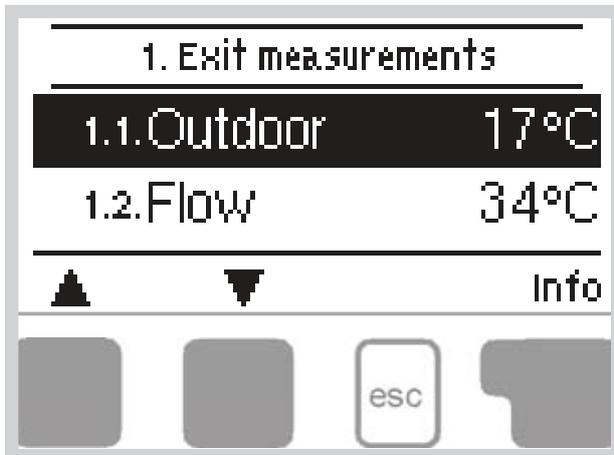
Menu „**1. Measurements**” serves to display the currently measured temperatures.
