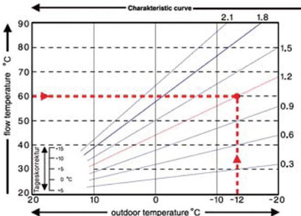
The diagram shows the influence of the selected characteristic curve steepness (standard curve) on the calculated reference flow temperature of the heating circuit. The correct curve is appointed by setting the intersection point of the calculated maximum flow temperature and the minimum outdoor temperature.
