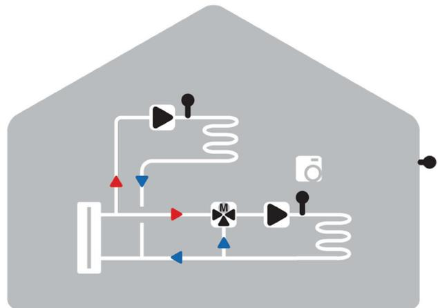
**5. Two heating circuits - mixed and direct one, with boiler, no accumulation tank**
