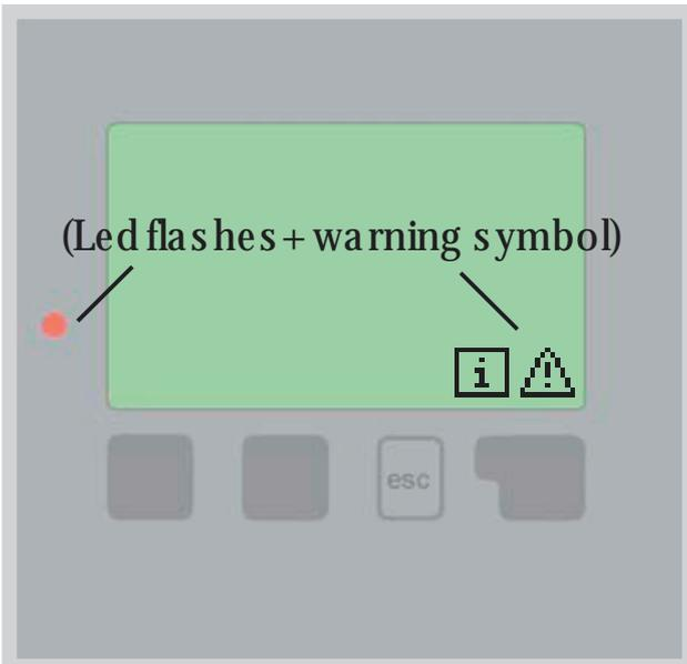
If the controller detects a malfunction, the red light flashes and the warning symbol also appears in the display. If the error is no longer present, the warning symbol changes to an info symbol and the red light no longer flashes.
