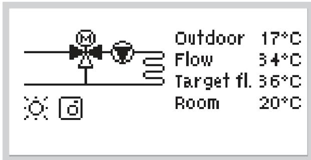
The graphics or overview mode appears when no key has been pressed for 2 minutes, or when the main menu is exited by pressing „**esc**”.
