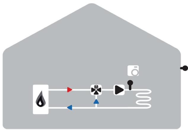
**3. Mixed heating circuit with boiler and accumulation tank**
