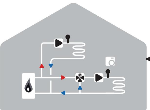
**6. Two heating circuits - mixed and direct one, with boiler and accumulation tank**
