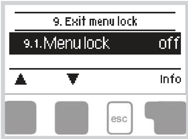
Menu „**9. Menu lock**” can be used to secure the controller against unintentional changing of the set values.
