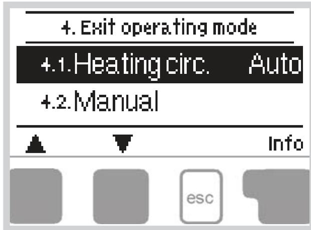
Menu „4. Operating mode” is used to specify the operating modes for the heating circuit. After an interruption of the mains voltage the controller automatically returns to the last operating mode selected!
