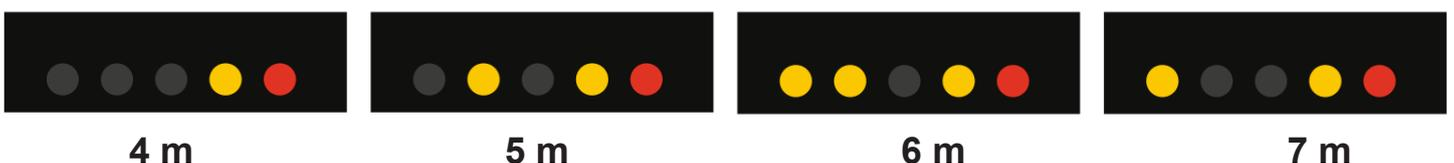
3. Release the button for more than 10 s and the LEDs will return to „performance view“, while the last setting is saved.
