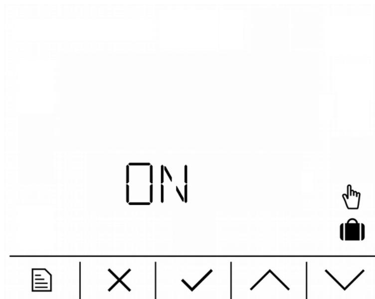
Holidays switch-on display. If not in edit mode, the display shows the current state of the Holiday function (**ON/OFF**); on entering the edit mode (pressing the OK key - the edit symbol starts flashing) the state can be changed.
