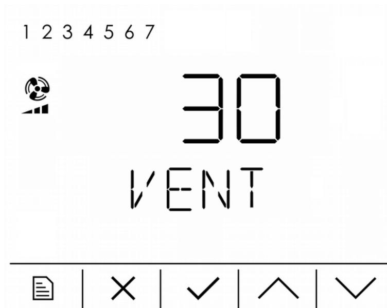
**Main value**                      Time period (in minutes) when the immediate ventilation function will be on. The power to which the ventilation unit fan will be set has to be changed in the controller's web interface.
