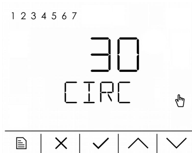
**Main value** Time period (in minutes) when the immediate recirculation function will be on.
