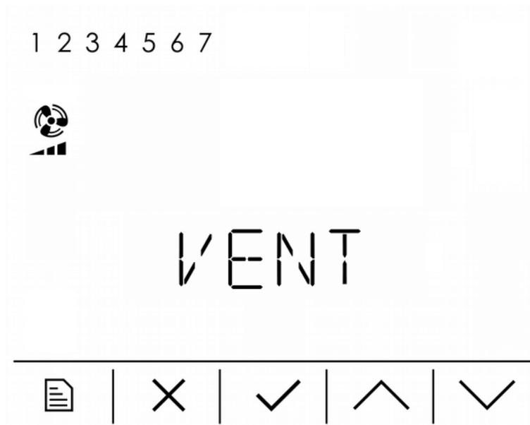
**Secondary value**      **VENT** text and the info on the immediate ventilation function on are displayed alternately (**ON/OFF**).
