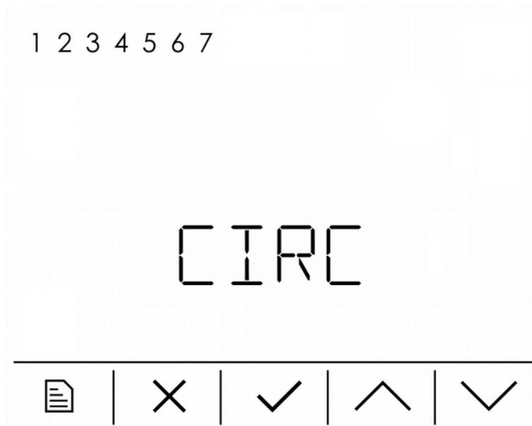
**Secondary value** *CIRC* text and the info on the immediate recirculation function on are displayed alternately (**ON/OFF**).
