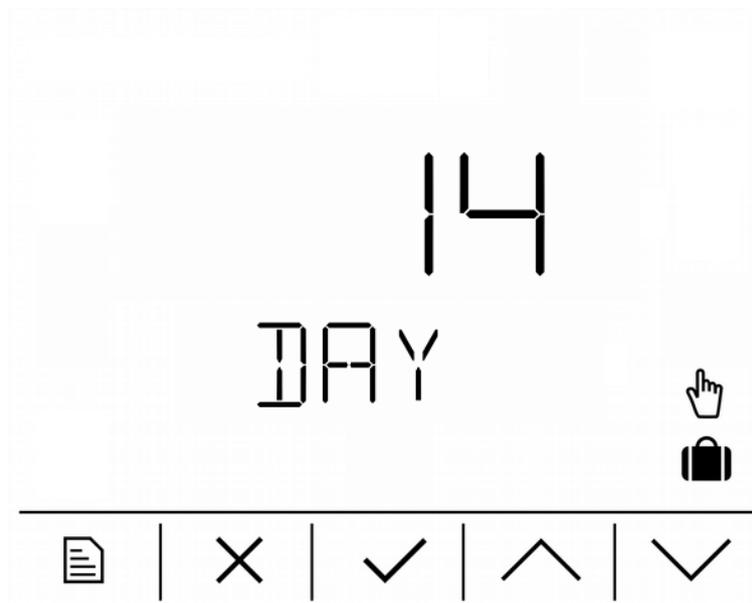
Setting how long (in days) the function shall be active when switched on. After the time expires, the function will be switched off.
