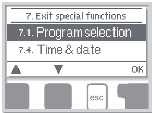
Menu „7. Special functions” is used to set basic items and expanded functions. Other than the time all settings may only be made by a specialist.
