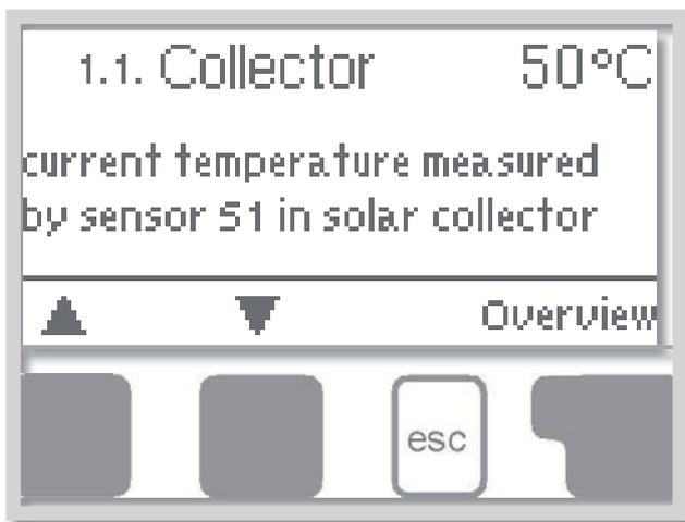
Selecting „**Details**” leads to a brief help text explaining the measurement values. Selecting „**Overview**” or „**esc**” exits the Info mode.
