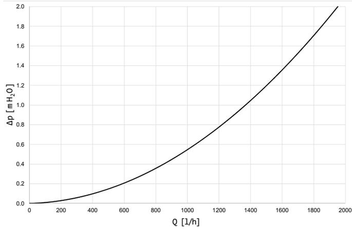
**Pressure drop diagram of RegulusHBOX K unit
