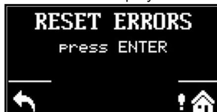
After pressing the button under the exclamation mark, faults will be displayed in this order: on pos. 1-3 heat pump faults, on pos. 4-5 other faults. On position 6 there is a screen for reset of heat pump faults.
