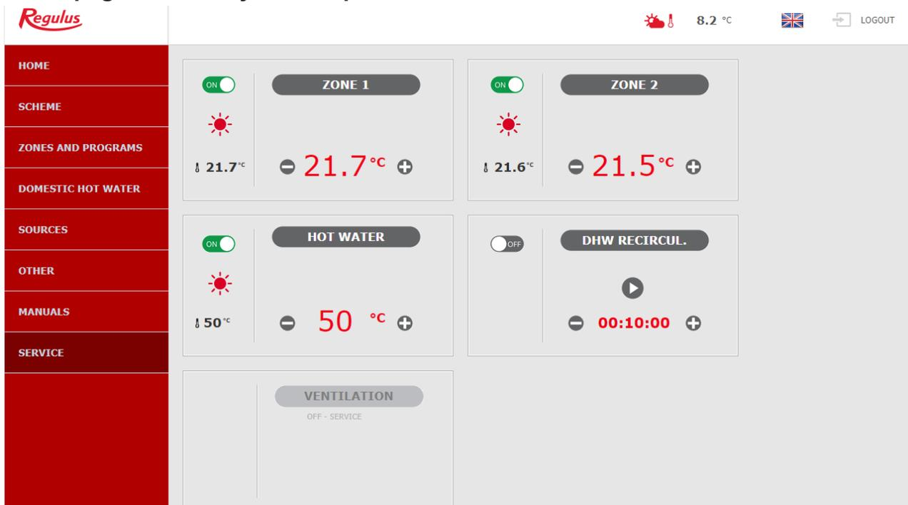
In the left part of the screen there is a menu to enter the individual sections for settings, at the top right there is a button for logging out of the web interface and a flag, allowing to change the language version of the web interface. When editing values (numbers, texts), it is necessary to confirm the change after each change by pressing the **SAVE CHANGES** button.
