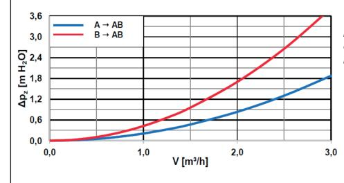
The pressure drop value moves between the two curves depending on the mixing ratio during mixing.
