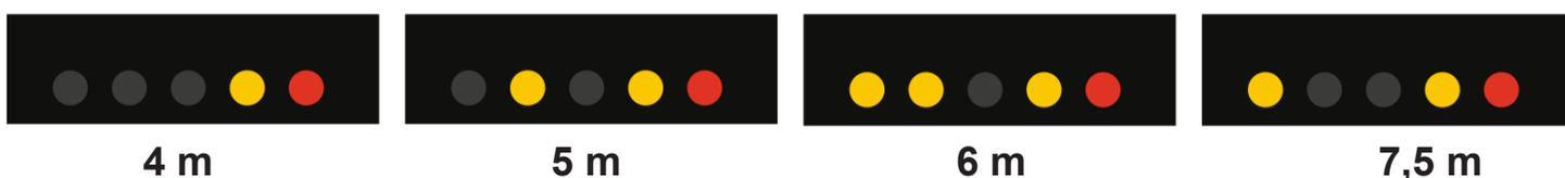
3. Release the button for more than 10 s and the LEDs will return to „performance view“, while the last setting is saved.
