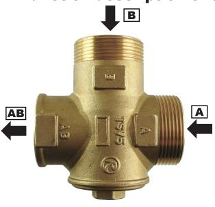
TSV5BMF 6/4Mx5/4F load valve is fitted with an integrated thermostatic insert that will close the **A** inlet (from a heating system), if the return water temperature to the boiler (**AB** outlet) is lower than the opening one. As soon as the opening temperature is reached, the thermostat starts opening the **A** inlet slowly and mixing the cold return water with the hot water from the boiler flow (**B** inlet) with the aim to reach the opening temperature in the return pipe (**AB** outlet).
