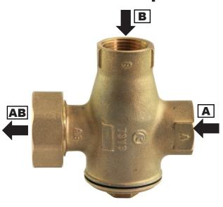
TSV3B load valve is fitted with an integrated thermostatic insert that will close the "A" inlet (from a heating system), if the return water temperature to the boiler ("AB" outlet) is lower than the opening one. As soon as the opening temperature is reached, the thermostat starts opening the "A" inlet slowly and mixing the cold return water with the hot water from the "B" inlet (boiler flow) with the aim to reach the opening temperature ("AB" outlet) in the return pipe.
