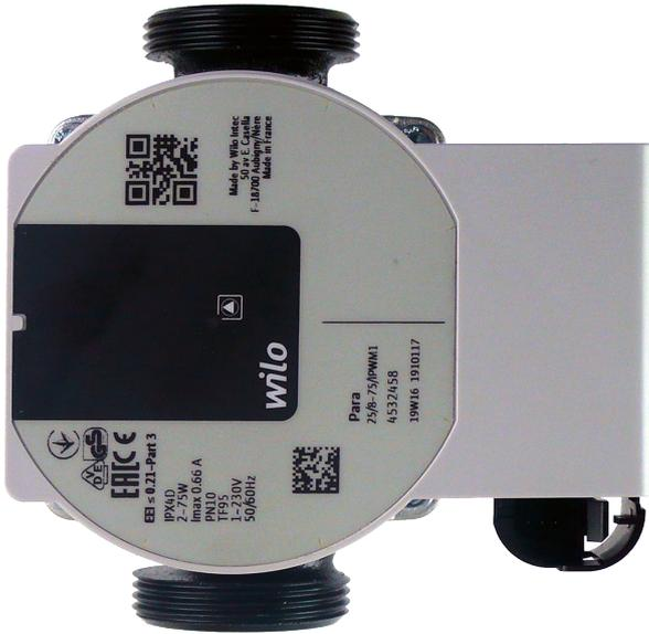
The Wilo Para 25/8 iPWM1 is a wet running circulation pump. The pump speed is controlled by the PWM signal. When the PWM signal is disconnected, the pump runs at its maximum speed. The operating status and possible faults of the pump are indicated by LEDs directly on the pump. The pump is able to send the current flowrate electronically to an external controller. The controller must be equipped with an iPWM read input and a flow calculation function.
