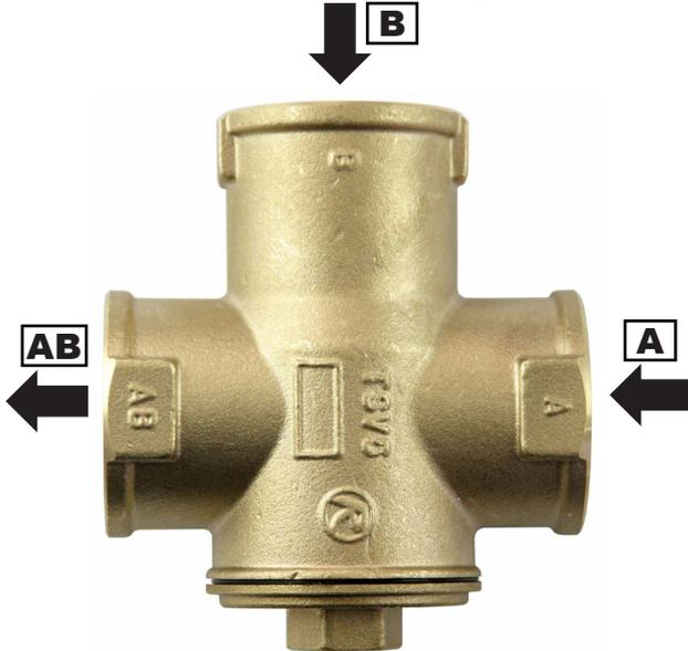
The TSV5B load valve is fitted with an integrated thermostatic insert that will close the **A** inlet (from a heating system), if the return water temperature to the boiler (**AB** outlet) is lower than the opening one. As soon as the opening temperature is reached, the thermostat starts opening the **A** inlet slowly and mixing the cold return water with the hot water from the **B** inlet (boiler flow) with the aim to reach the opening temperature (**AB** outlet) in the return pipe.
