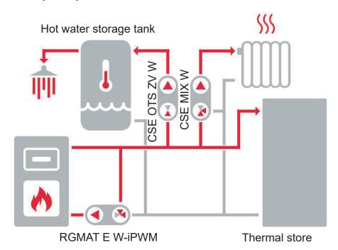
The diagram shows a typical connection of a solid fuel boiler, thermal store and heating circuit (with the recommended CSE MIX W pump station – not included in supply). If the boiler is used also for hot water heating, it is recommended to install a CSE OTS ZV W pump station (not included in supply).
