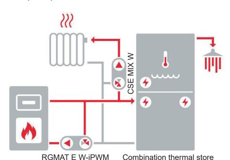
The diagram shows a typical connection of a solid fuel boiler, combination thermal store and heating circuit (with the recommended CSE MIX W pump station – not included in supply).
