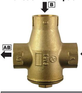
The TSV3B load valve is fitted with an integrated thermostatic insert that will close the **A** inlet (from a heating system), if the return water temperature to the boiler (**AB** outlet) is lower than the opening one. As soon as the opening temperature is reached, the thermostat starts opening the **A** inlet slowly and mixing the cold return water with the hot water from the **B** inlet (boiler flow) with the aim to reach the opening temperature (**AB** outlet) in the return pipe.
