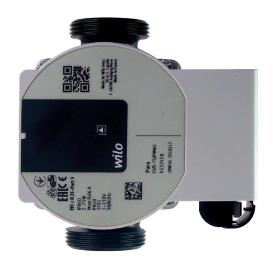
The Wilo Para 25/8 iPWM1 is a wet running circulation pump. The pump speed is controlled by the PWM signal. When the PWM signal is disconnected, the pump runs at its maximum speed. The operating status and possible faults of the pump are indicated by LEDs directly on the pump. The pump is able to send the current flowrate electronically to an external controller. The controller must be equipped with an iPWM read input and a flow calculation function.
