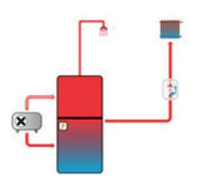
The accessories consist of a thermal store for heating only (Regulus PS series), or a combination thermal store with immersed DHW tank (Regulus DUO series), or a thermal store with stainless steel tube DHW exchanger (Regulus HSK series). TThis connection is suitable for combining a heat pump with
