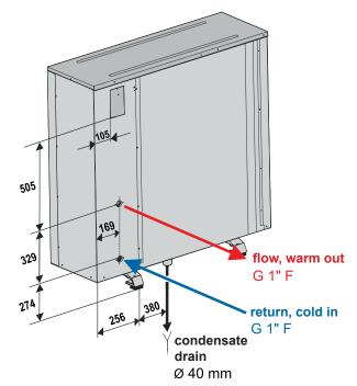
pump using braided diffusion-tight hoses of suitable length. Hoses are included in the delivery only for heat pumps supplied as a Special Offer, otherwise they must be ordered separately. Braided diffusion-tight hoses with F/F or M/F threads for RTC 12i heat pumps can be ordered in lengths of 500, 700 and 1000 mm. To eliminate the transmission of vibrations to the adjoining pipeline and possibly also to the house structure, it is recommended to run the braided hose loose in a slight bend.
