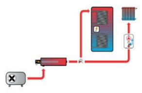
In this direct connection to the heating system, it is necessary to keep the minimum flow through the heat pump at the level of min. **790** I/h with sufficient heat supply for defrosting, i.e. it is necessary to have a part of the heating system without shut-off valves installed, e.g. thermostatic valves. Approximately it is at least 5 radiators of normal size (e.g.  $0.6 \times 0.9 \text{ m}$ ), or at least 30 m<sup>2</sup> of underfloor heating without the possibility to be shut off.
