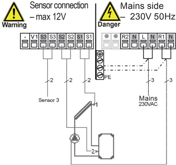
Relays R1 and R2 switch at the same time in this wiring, so the pump can be wired to R2.
