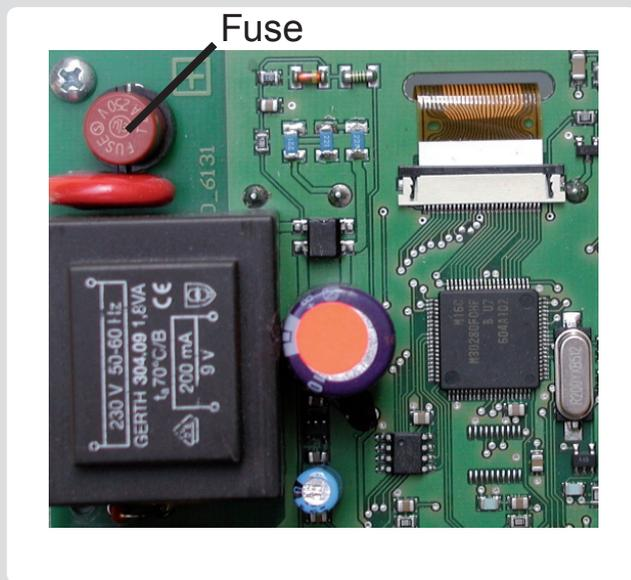
If the mains voltage is switched on and the controller still does not function or display anything, then the internal device fuse may be defective. In that case, disconnect the device, open it, remove the old fuse and check it. Replace the defective fuse with a new one, locate the external source of the error (e.g. pump) and replace it. Then first re-commission the controller and check the function of the switch outputs in manual mode as described in Chap. 4.2.
