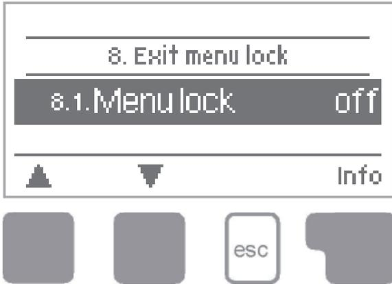
Menu “8. Menu lock” can be used to secure the controller against unintentional changing of the set values.
