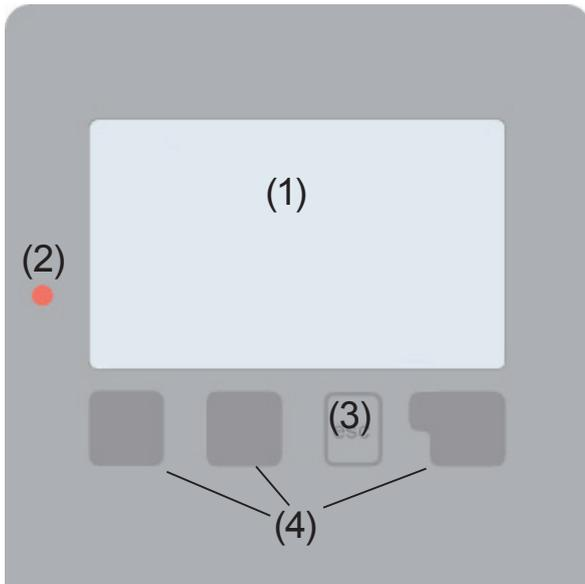
The display (1) shows graphic and text info on the hydraulic variant, set and measured values and other text info.
