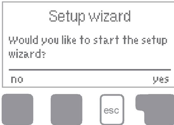
The first time the controller is turned on, language and clock need to be set. After that a query appears as to whether you want to parameterize the controller using the commissioning help or not. The commissioning help can also be terminated or called up again at any time in the special functions menu. The commissioning help guides you through the necessary basic settings in the correct order,
