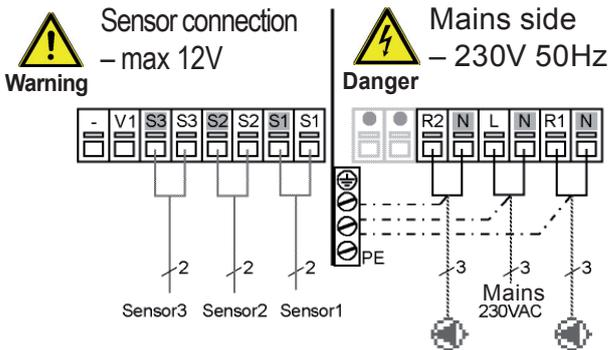
Controller switching function: If the temperature at S1 exceeds that at S2, the R1 pump relay will close.
