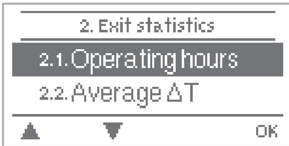
Menu “2. Statistics” is used for function control and long-term monitoring of the system.
