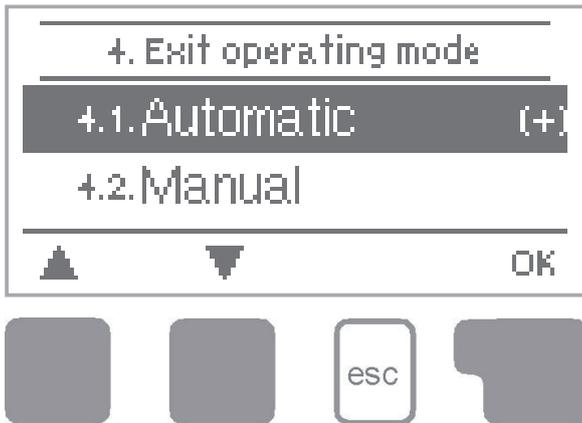
In menu “4. Operation mode” the controller can either be switched to automatic mode, switched off, or switched to a manual operating mode.
