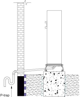
It is recommended to insulate the outdoor section of drain pipe with thermal insulation.
