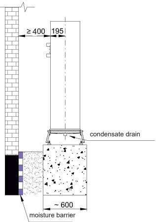
Water condensation normally occurs during heat pump operation; up to 50 liters of condensate can be generated per day, depending on the operating conditions.
