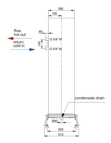
Compensators (included in supply) shall be fitted to the heat pump connecting pipes (G 5/4" M) to increase the frost protection of the plate heat exchanger of the heat pump.
