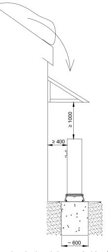
Avoid using materials with increased sound reflectivity near the device; it is unsuitable, for example, to line the surrounding surfaces with ceramic tiles.
