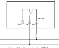
Wiring of the thermostat for RT3E.
