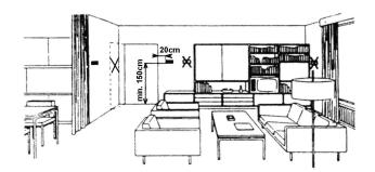
This thermostat is intended for indoor use only. It should be mounted on an inner wall, about 150 cm above the floor, located where room temperature changes can be felt thanks to freely circulating air.
