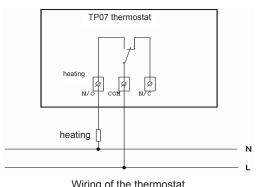
Wiring of the thermostat
