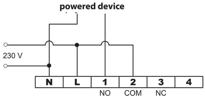
The voltage at terminals 1 and 2 depends solely on the system to be controlled, so the cable cross-section must respect the type of device controlled by the thermostat. The length of the cables does not play any role, the receiver can be placed near the boiler or far from it, but never under its casing.
