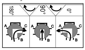
PERMISSIBLE HYDRAULIC CONNECTION (VALVE INSTALLED AS A FLOW DIVIDER)
