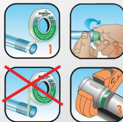
The joint permits a position shift of the components. Should the threaded joint come loose, it can be re-tightened. Do not apply excessive amount of the tape as the surplus could be squeezed out of the thread.
