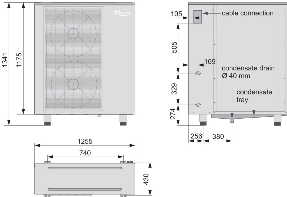
**RTC 12i Air-to-water Heat Pump**
