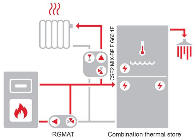
The diagram shows a typical connection of a solid fuel boiler (with the recommended RGMAT pump station – not included in supply), combination thermal store and heating circuit.
