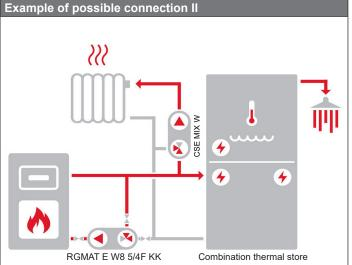
The diagram shows a typical connection of a solid fuel boiler, combination thermal store and a heating circuit (with the recommended CSE MIX W pump station – not included in supply).
