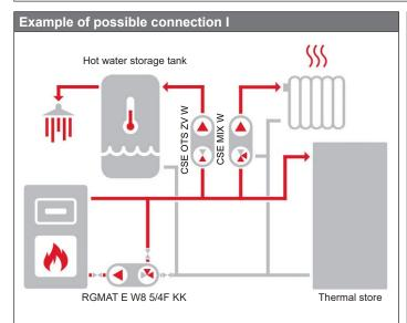
The diagram shows a typical connection of a solid fuel boiler, thermal store and heating circuit (with the recommended CSE MIX W pump station – not included in supply). If the boiler is used also for hot water heating, it is recommended to install a CSE OTS ZV W pump station (not included in supply).
